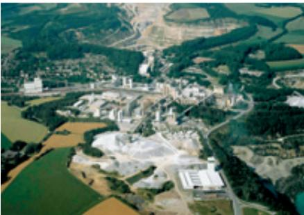
some 8 million tons of limestone in their Flandersbach plant each year and use it to produce 1.8 million tons of burned and more than 3 million tons of un-burned lime products.
